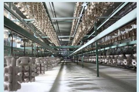
Auto-drying system for casting
